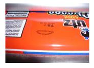
Thermal transfer overprinters feature a printhead and ribbon that make contact with a flexible substrate and create real-time images, including clean, high-resolution bar codes, text and graphics. For Utz, any product coding machine has to be robust enough to handle high line speeds while producing consistently readable codes. That was not the case with Utz's hot stampers, and also one of the reasons Epley first brought in thermal transfer printers.
